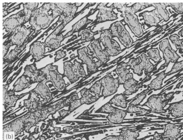
Figure 3 Microstructure of basic Fe-C-Cr-V alloy containing 2.02% V: (a) as-cast; (b) heat-treated 500°C/4 h (magnification \times 390 ).
